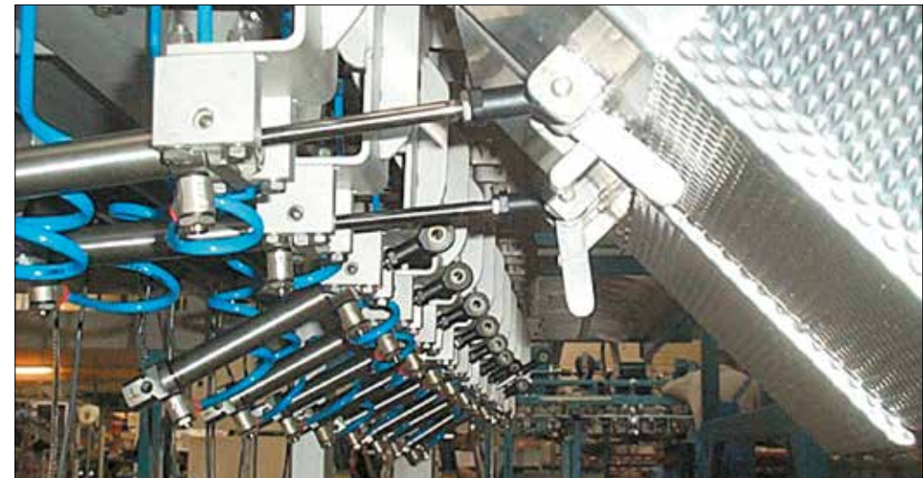
igubal® spherical bearing in pneumatically driven flap bearing.
