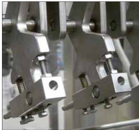
Maintenance-free iglidur® X6 plain bearings are used in the toggle lever systems that grab onto the bottles.
