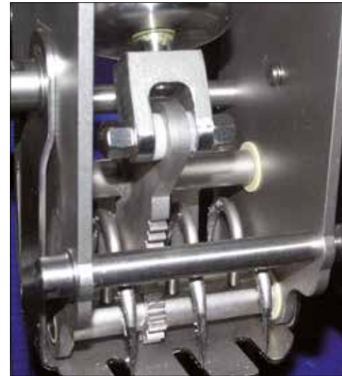
Mounting of the holder of the material to be cut in tray and fork design. It is driven by a pneumatic cylinder for implementing the pivoting movement with iglidur® J plain bearings.
