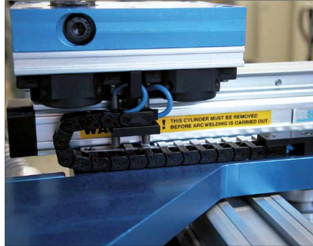
Even for the narrowest installation space – bending radii from 4 \times d with e-chains® and chainflex®.
