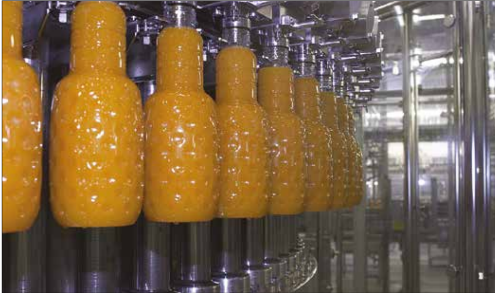
Pneumatic lifting device for filling machines – iglidur® H370 gives you a low coefficient of friction in dry operation, chemical resistance and low moisture absorption.
