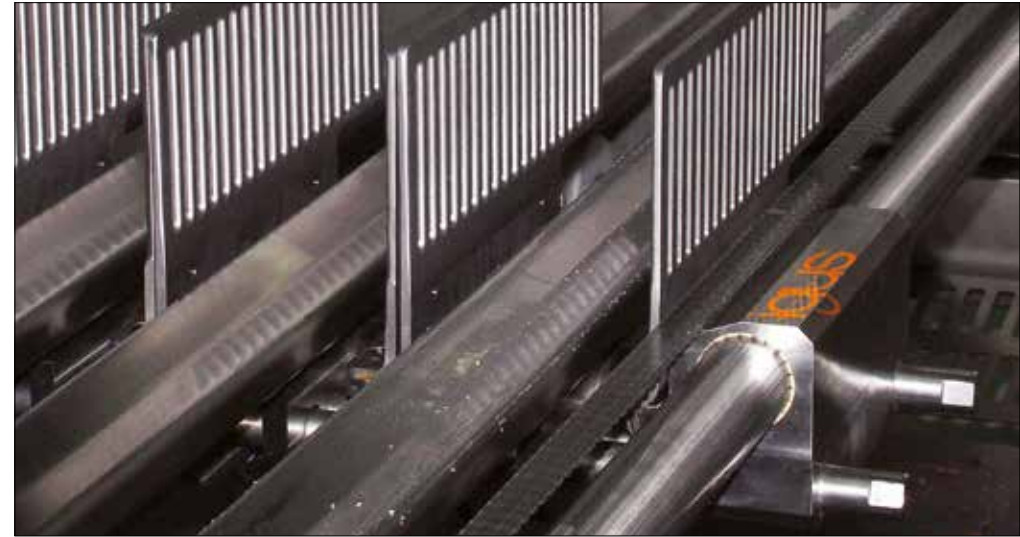
Linear stroke of the pre-gripper for feeding the material to be cut. Thereby soft stainless steel shafts and linear films of the type series drylin® JUM-01-40 are used.
