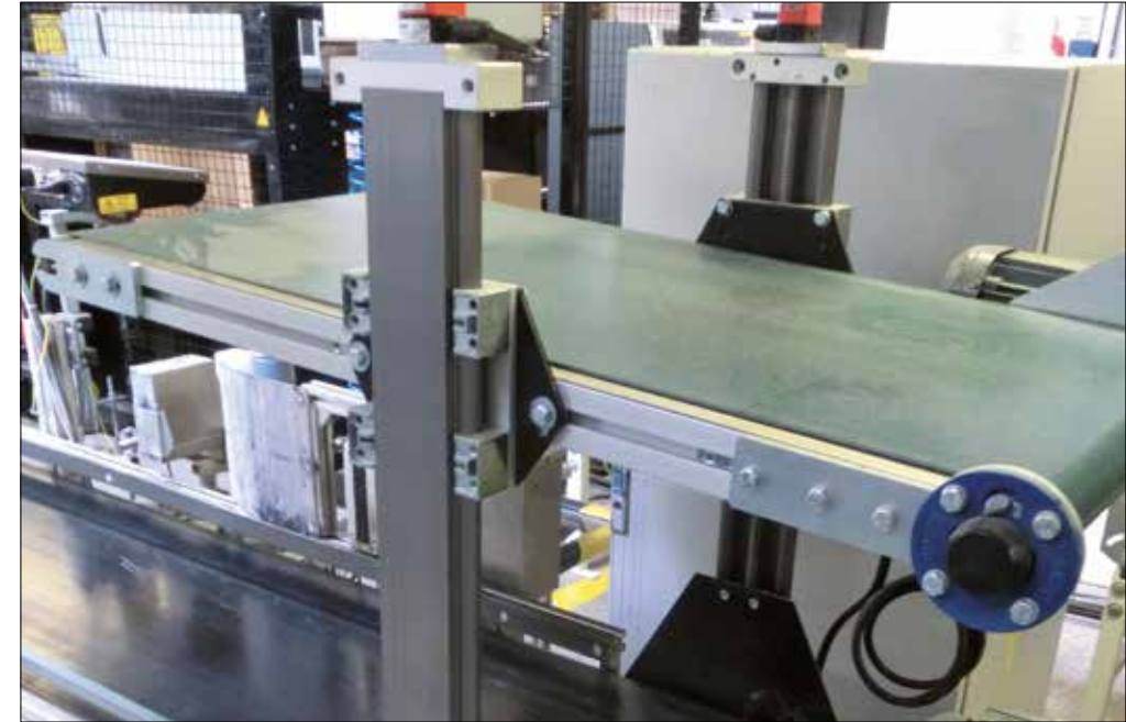
drylin® SLW-2080 lead screw units provide the synchronised height adjustment for pressing the packed diapers into cartons.
