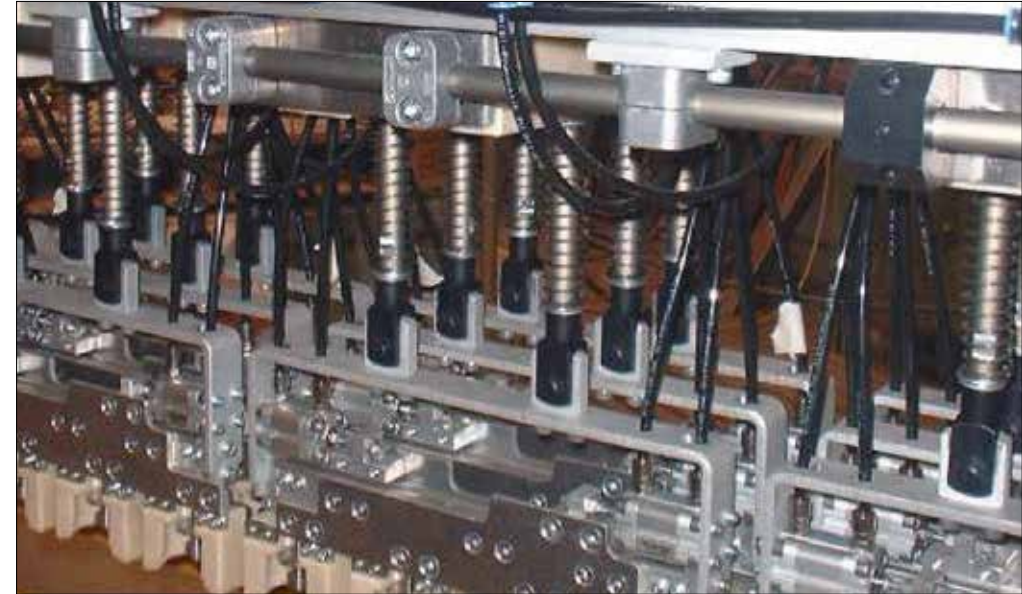
Bottle packing machine: The redevelopment of a gripper using igus® plain bearing elements resulted in a very thin, rugged and Lubrication-free gripper tool that is right now not available in the market.
