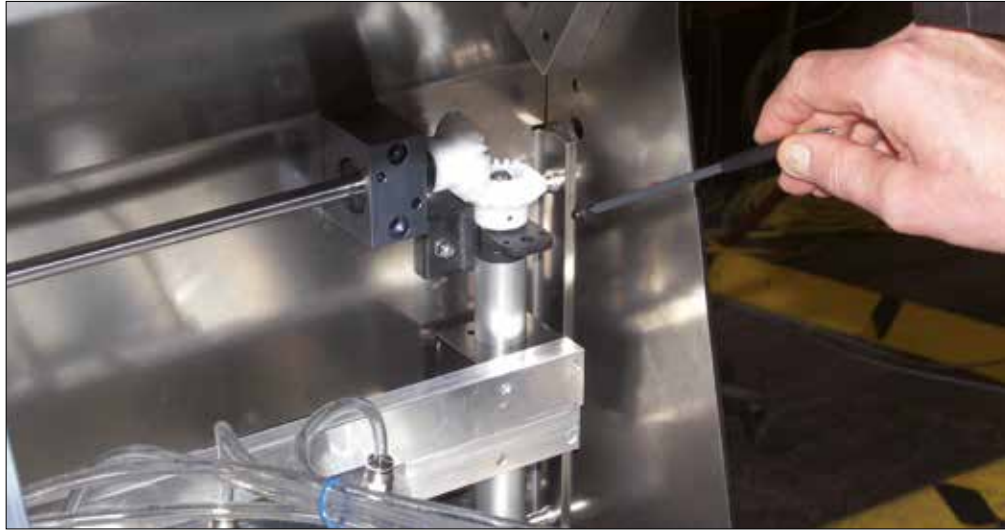
Adjustment and format adjustment of a prism beam in the stripping station of ice cream cones using drylin® easytube SET-25-AWM.
