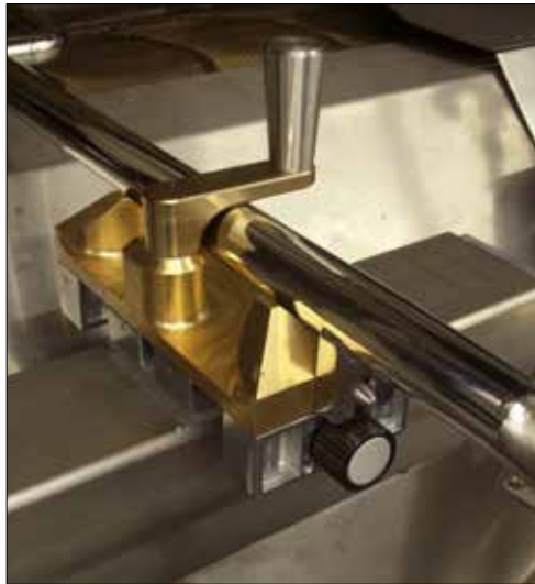
Position adjustment of the batter spray pipe with a clearance-adjustable drylin® SLW-1040 lead screw unit.
