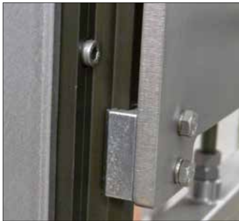
drylin® W linear guide systems are used in the neck sleeve removers. These are also maintenance-free and resistant against cleaning agents used by the beverages industry.
