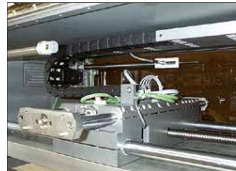
Even for the narrowest installation space – bending radii from 4 \times d with e-chains® and chainflex®.
