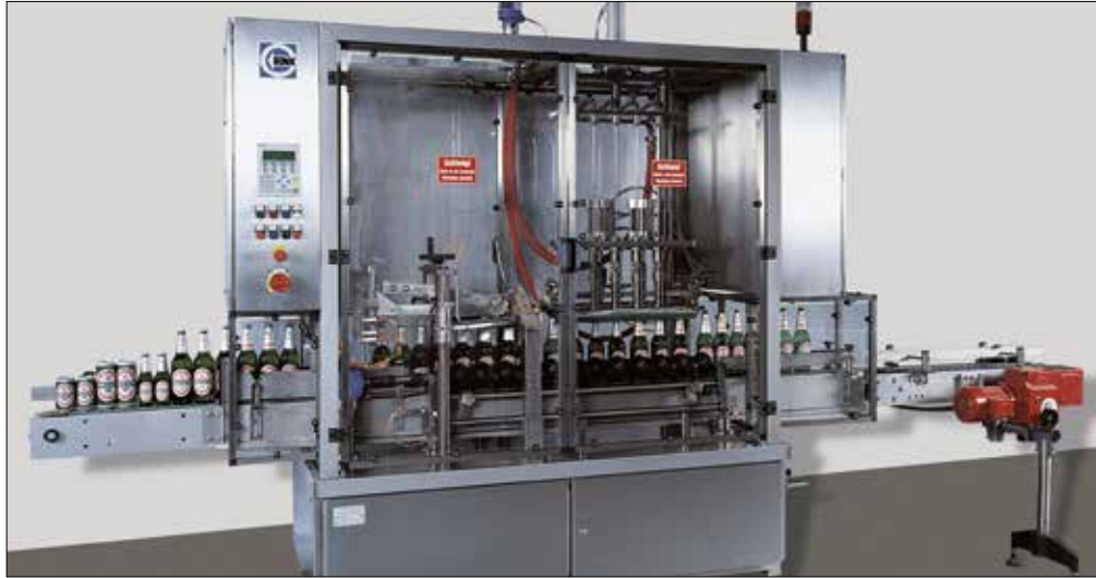
Automatic plant for bottle emptying. The valves on this plant are equipped with cylindrical drylin® linear bearings.
