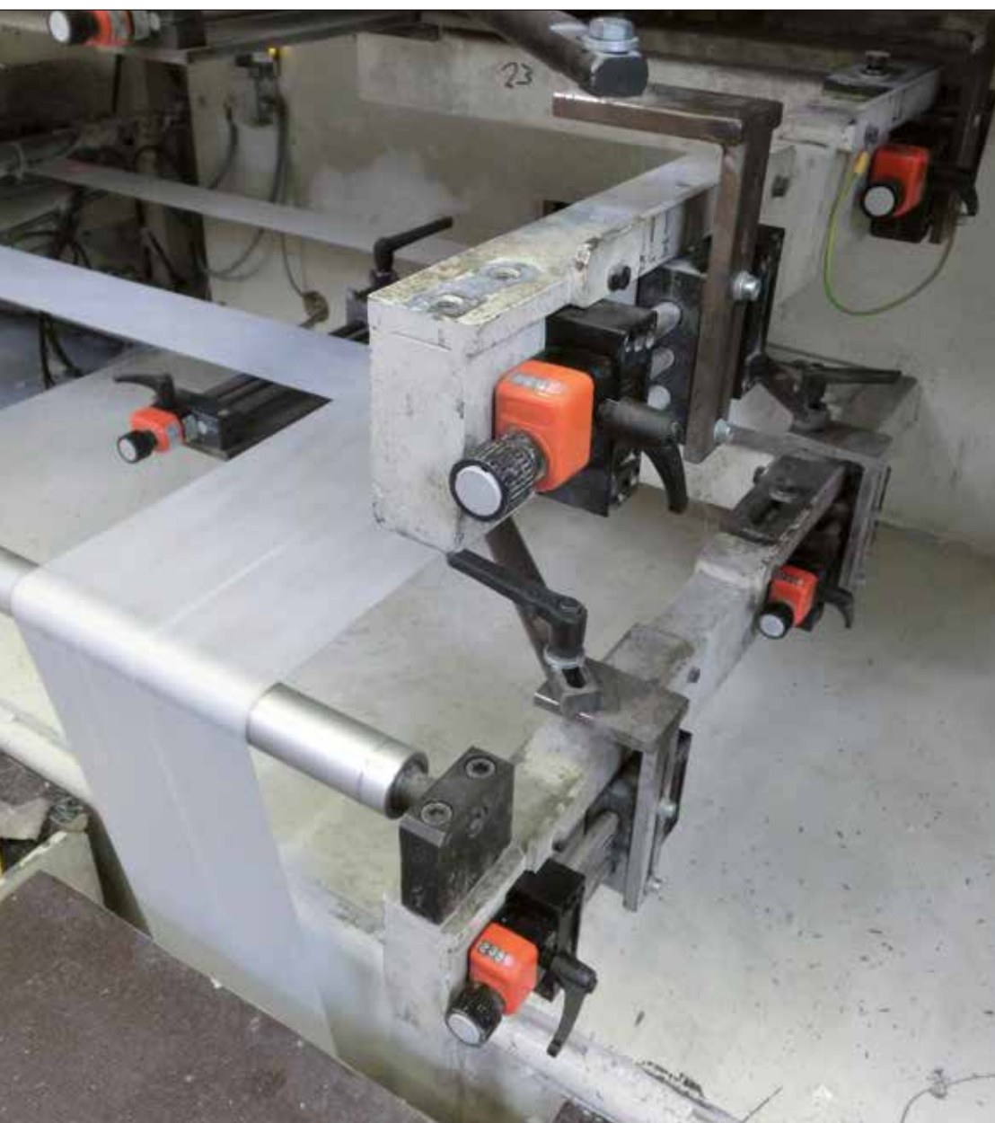
Middle adjustment of a four-web 90° deflection using drylin® lead screw unit SHT-12-AWM for non-woven webs. A total of eight systems are in use.
