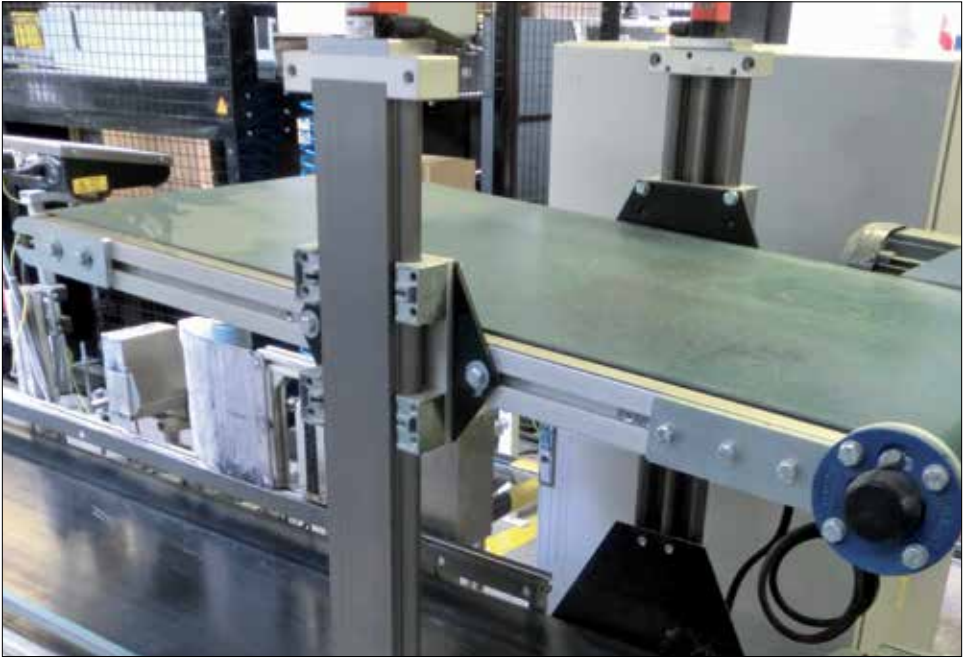
drylin® SLW-2080 lead screw units provide the synchronized height adjustment for pressing the packed diapers into cartons.
