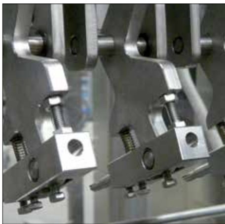
Maintenance-free iglide® X6 bearings are used in the toggle lever systems that grab onto the bottles.
