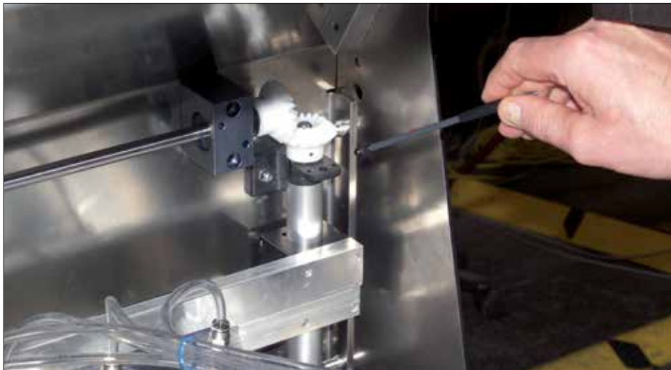
Format adjustment of a prism beam in the stripping station of ice cream cones using drylin® Easy Tube SET-25-AWM.
