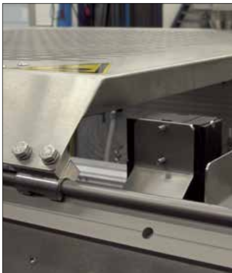
Safety adjustment with maintenance-free drylin® WJRM hybrid bearings for the lowest adjustment forces.
