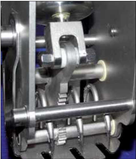
Mounting of the holder of the material to be cut in tray and fork design. It is driven by a pneumatic cylinder for implementing the pivoting movement with iglide® J bearings.
