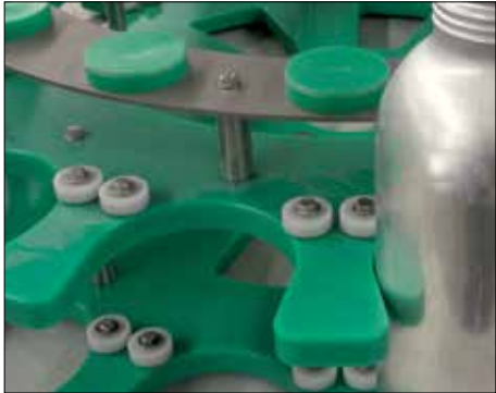
The xiros® plastic ball bearings are used in a series of packaging machines. Sturdy and smooth, they often replace more expensive metallic roller bearings.
