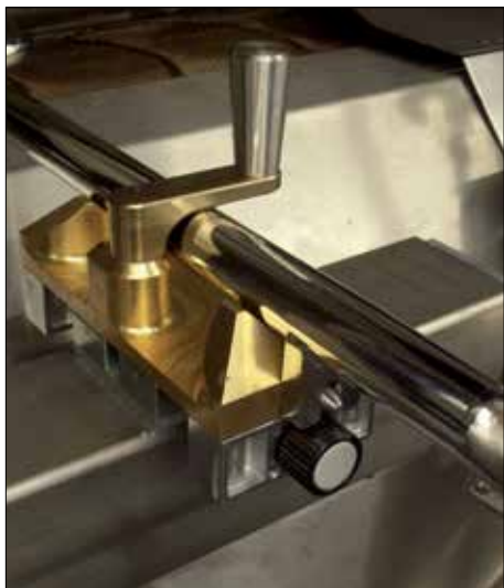
Position adjustment of the batter spray pipe with a clearance-adjustable drylin® SLW-1040 lead screw unit.
