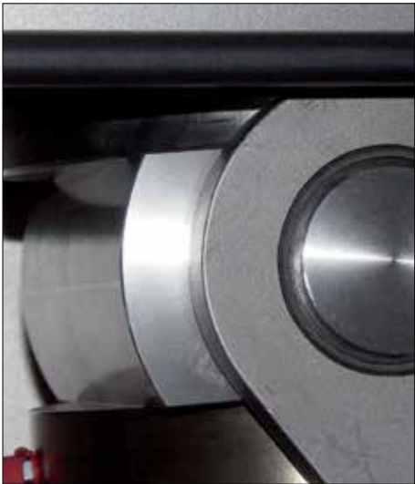
Pivotal mounting of the feed arm with iglide® X6 bearings.
