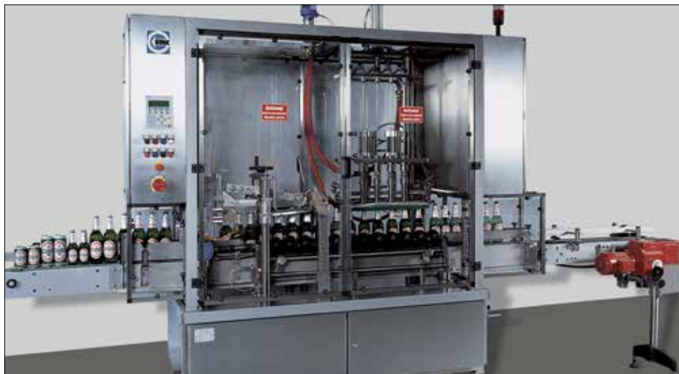
Automatic plant for bottle emptying. The valves on this plant are equipped with cylindrical drylin® linear bearings.
