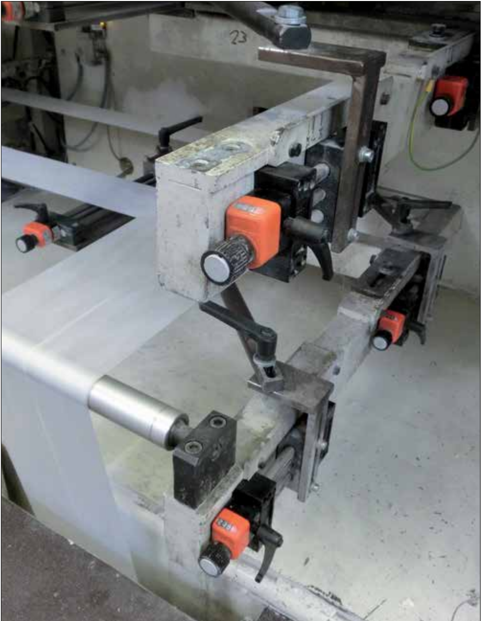
Middle adjustment of a four-web 90° deflection using drylin® lead screw unit HTS-12-AWM for non-woven webs. A total of eight systems are in use.
