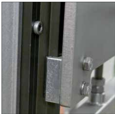
drylin® W linear guide systems are used in the neck sleeve removers. These are also maintenance-free and resistant to cleaning agents used by the beverage industry.
