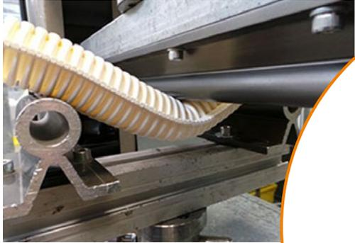
Bending test on the e-skin® soft corrugated tube
