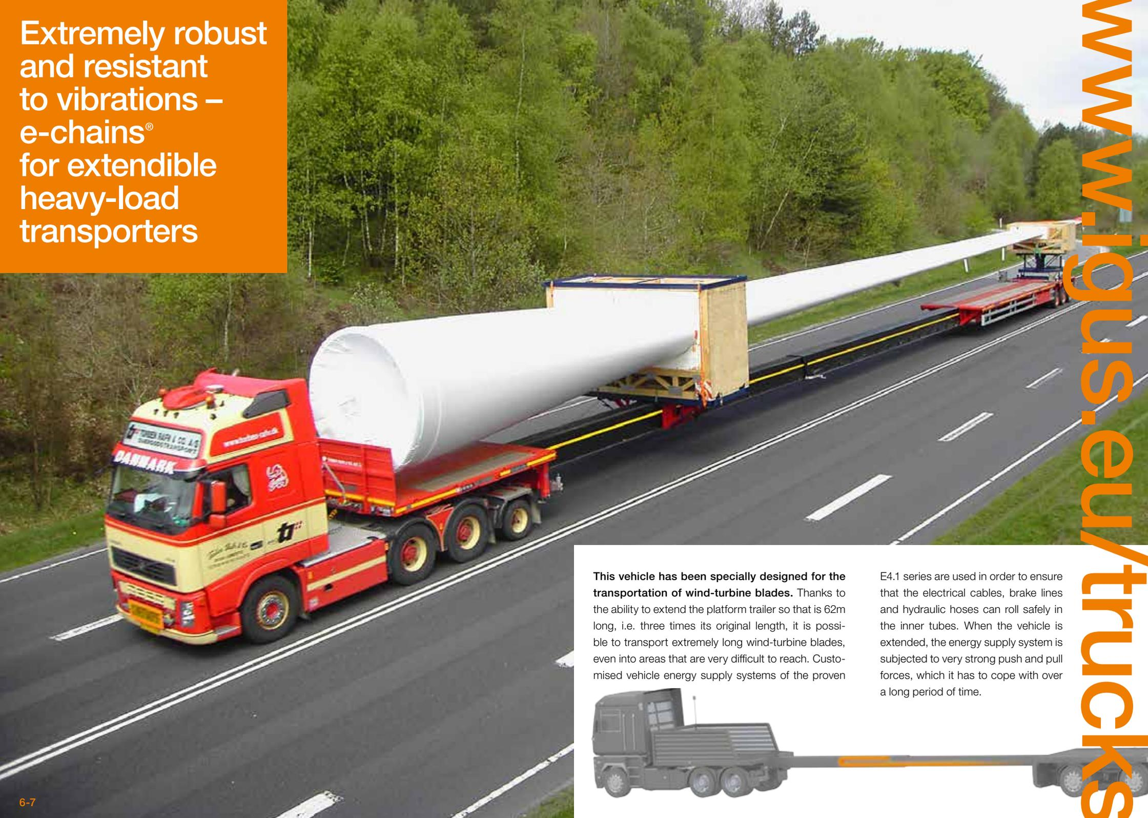
**This vehicle has been specially designed for the transportation of wind-turbine blades.** Thanks to the ability to extend the platform trailer so that is 62m long, i.e. three times its original length, it is possible to transport extremely long wind-turbine blades, even into areas that are very difficult to reach. Customised vehicle energy supply systems of the proven
